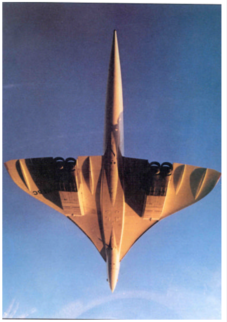
An impressive sunlit underside, highlighting the elegant delta wing, under-slung engines and elongated tail.
